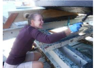
Charlie's Chariot has been anti-fouled and the engine serviced.
